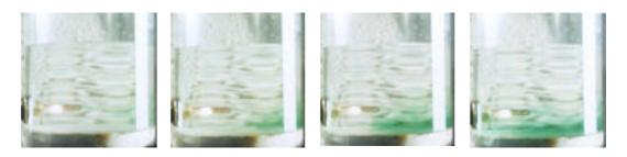
The results from the circulating jet again fell on a straight line through the origin but the coefficient of stratification of 0.65 was significantly lower than a straight horizontal jet. The results are plotted in figure 4.9.
