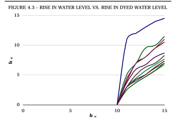
If this was the case, all mixing would be occurring well below the mixing front and there would be no further mixing of clear water as the height of the clear water ( $h_{o}$ ) would remain constant (see figure 4.4)., For this reason the height of the water level was subtracted from the height of the dyed water mixing front, leaving only the height where actual mixing was taking place ( $h_{m}$ ).
