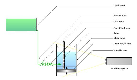
The nozzle arrangement was a standard plumbing fitting into which either different sized inserts or a number of different nozzle configurations made from copper pipe could be fitted. Measurements were taken by siting across two rulers and each trial was timed with a stopwatch.
