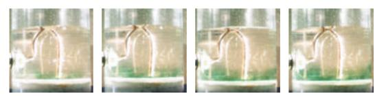
Once again the results fell on straight lines however the coefficients of stratification ranged as the height of the nozzle changed. The resultant coefficients are in table 4.2. The actual results are graphed in figure 4.12 The results for central positioning and positioning next to the wall fall on the same line. So mixing appears insensitive to the horizontal placement of
