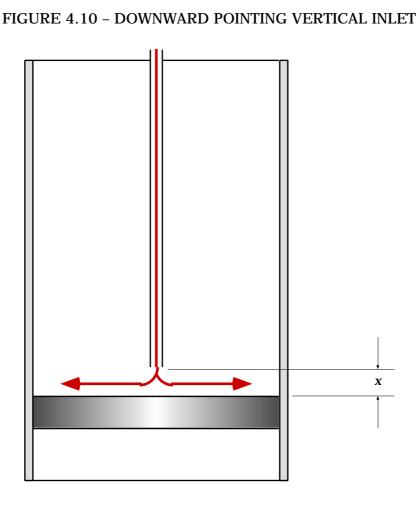
Tests were made with the inlet at several heights above the base (*x*), centrally and near to the tank wall
