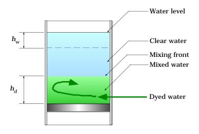
Each test was timed and the total volume discharge (A  $h_w$ ) was divided by the test time to obtain the velocity of the jet. The temperatures and salt quantities were used to calculate the buoyancy. The densimetric Froude number was then calculated from these values and the jet diameter.
