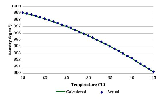
FIGURE 3.3 – DENSITY OF WATER VS. TEMPERATURE
