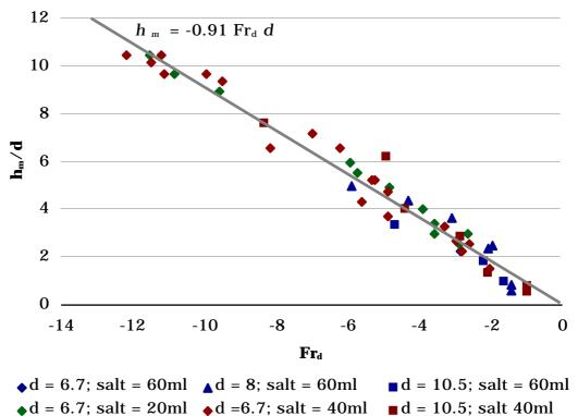
This relation appears robust against changes in diameter, discharge, buoyancy and water level so the results should be scaleable.
