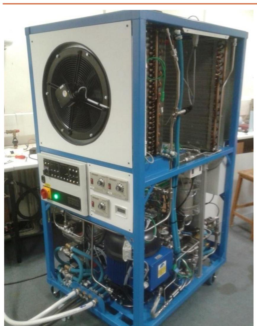
8 kW cooling capacity prototype
