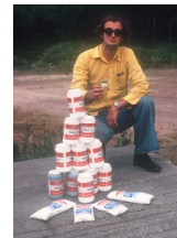
Comparative injection volumes of salt and fluorescein for a ground water test
