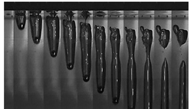
FIG. 8. Figure 28 from Tan (2016). The deep seal and shallow seal observed following the entry of a steel sphere ( D = 7 mm and u_i = 3.96 m/s) into sunflower oil. The cavity expanded while being dragged into the oil. The time difference between each of the successive images is 4 ms.
