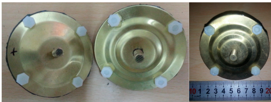
Figure 10. Two constructed transducers.
