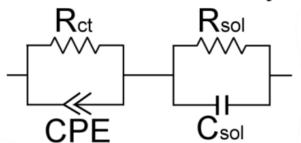
$$Z' = R_{sol} + R_{ct} \left( \frac{1 + R_{ct} Q \omega^{n} \cos(n\pi/2)}{1 + (R_{ct} Q \omega^{n})^{2} + 2R_{ct} Q \omega^{n} \cos(n\pi/2)} \right)$$
