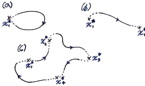
Figure 2.3: (a) A homoclinic orbit. (b) A heteroclinic orbit. (c) A heteroclinic cycle.
