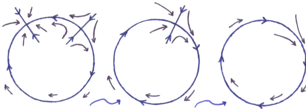
Figure 5.14: In the last stage of the bifurcation, the flow is slow near where the fixed point used to be and fast on the opposite side of the periodic orbit.
