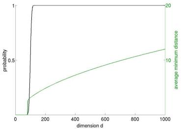
a projection neuron with *d* presynaptic inputs can separate almost any pair of trajectories that are each defined by connecting *less than d* randomly drawn points.
