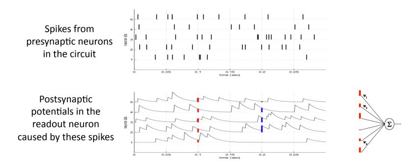
This high dimensional analog input is called the liquid state
