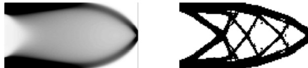
FIGURE 4. Plot of h'_\delta calculated with data as in Figure 3 but using a 240 \times 120 mesh. Note that the unregularized design on the right is mesh dependent. The discrete designs are also sensitive to the initial data and the fraction of elements allowed to change in each iteration. Although the discrete design here differs a lot from the one in Figure 3, the compliances only differs by less than 0.1 percent.
