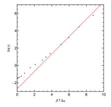
$\tau$  is the time for a single defect to move. Data from MD simulation of Bowles and Saika-Voivod, PRE **73**, 011503 (2006). Red line: transition state theory i.e. activated dynamics.
