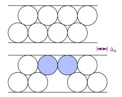
Upper Figure: the jammed state of maximum density.  $\phi_{max} = 0.8418$ .
