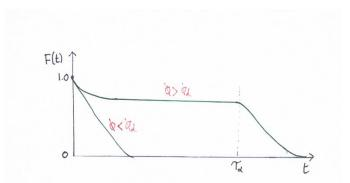
For  $\phi > \phi_d \approx 0.48$  (Bowles et al.) the time scales are long and activated  $\alpha_{\alpha}$
