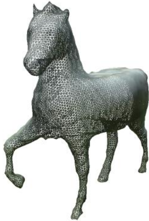
Fig. 16. Triangulated mesh of the reconstructed outdoor sculpture. This model was composed of 29,672 triangles.
