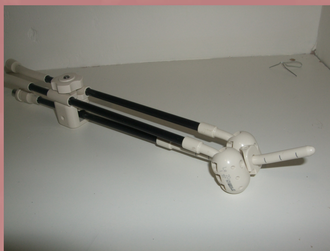
Figure 1: An MRI-safe version of the Manchester applicator
