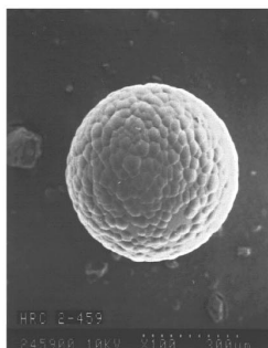
(a) Scanning electron microscope (SEM) image of “bumpy-ball” target surface \sigma = 1.7 \mu\text{m}
