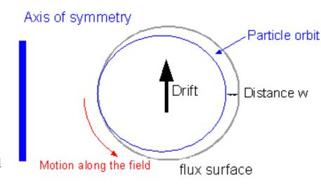
Due to the combined effect of the motion along the field line and the drift, the particle moves a finite distance (w) from the surface
