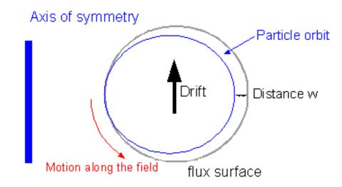
Due to the combined effect of the motion along the field line and the drift, the particle moves a finite distance (w) from the surface
