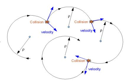
Collisional scattering leads to a random walk of the particle in space
