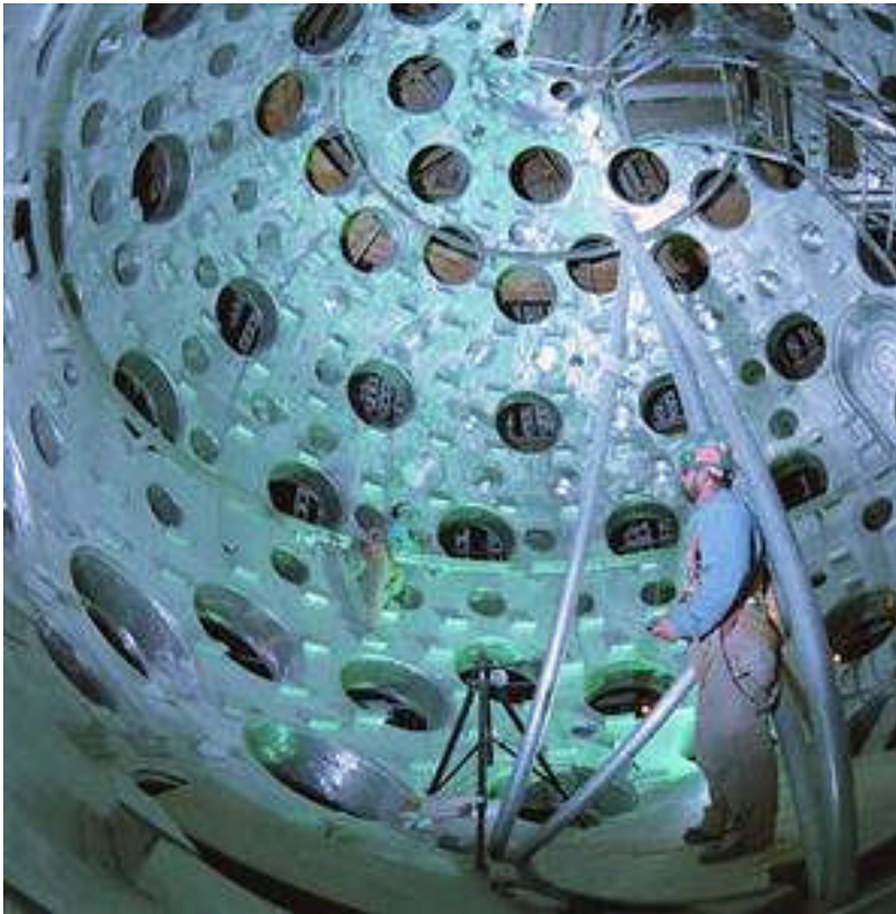
Target chamber, NIF with 192 laser beams
