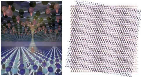
**Left figure:** A cartoon of "quantum tunnelling" of electrons (red balls with arrows) between a sheet of graphene (top layer, black atoms) and tungsten diselenide (bottom layer, dark and light blue atoms).
