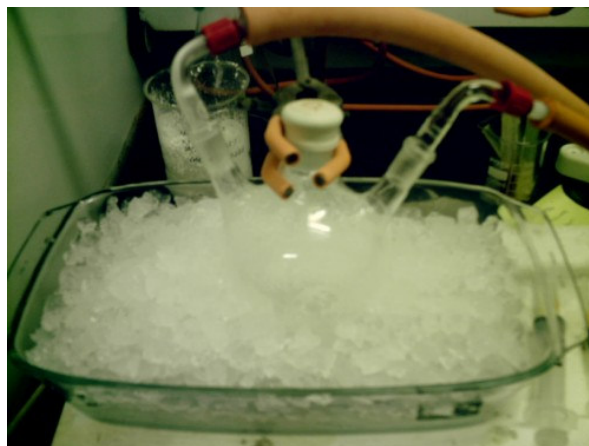
Figure 4.1 Arrangement used to prepare sol-gel silicon oxide powders, based on that used by Abys et al. [17]. Orange rubber tubes indicate the nitrogen in- and out-flow. Round-bottomed flask is sat in an ice bath, cooling the diethyl ether solvent, which is added to the flask prior to addition of water and silicon tetrachloride.
