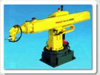
Polar robot is able to rotate in two different directions along his main axes and the third joint moves in translation forming a hemisphere or polar coordinate system.
