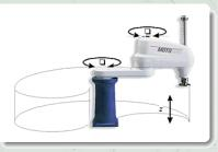
One disadvantage is that it can be more expensive because the controlling software requires inverse kinematics for linear interpolated moves. The work envelope of the SCARA robot tends to be difficult to control, and restricted in volume coverage.
