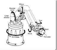
Motion from one point to another can be difficult to visualise as the robot will move each joint through the minimum angle required.
