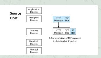
• The transport process passes the TCP segment down to the internet process, which encapsulates the segment in an IP packet.
