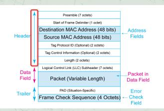
• The Ethernet frame has a header, data field, and trailer. The header has multiple fields.
