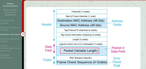
• The Ethernet data field contains the packet that the frame is delivering.
