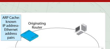
5. Originating router replaces IP-Ethernet address pair in ARP cache. Uses this address to send future frames to Host 10.19.8.17 without using ARP.
