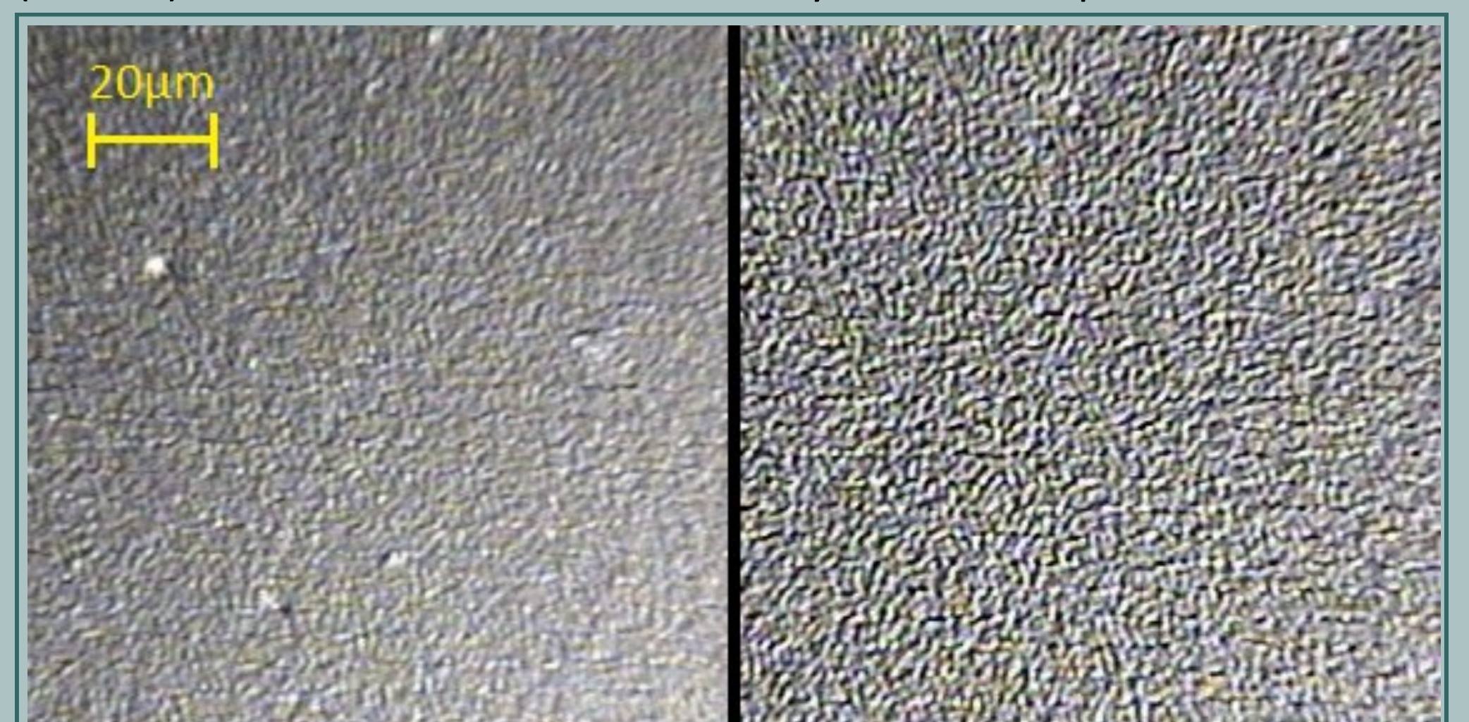
Fig 4: Optical images at 20x magnification of the roughened silicon surface having undergone 30 min (left) and 45 min (right) of the roughening process.
