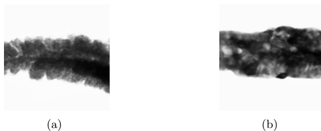
Figure 4.24: TEM images of the same part of the same AuPd nanowire (a) before and (b) after annealing. The images are 150 nm wide.
