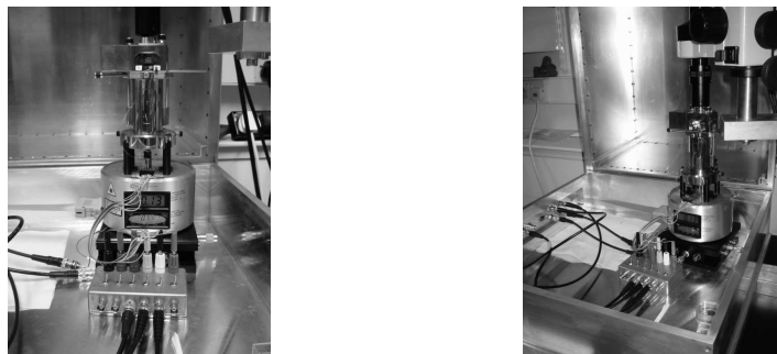
Figure 3.4: Experimental setup for multiple contact experiments on the Multimode AFM.
