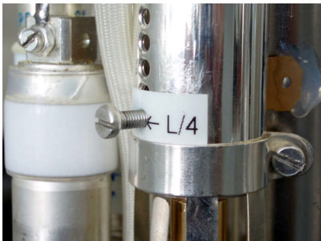
Fig.3 screw out \rightarrow \lambda/2 -mode
