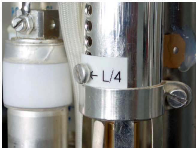
Fig.4 screw in \rightarrow \lambda/4 -mode
