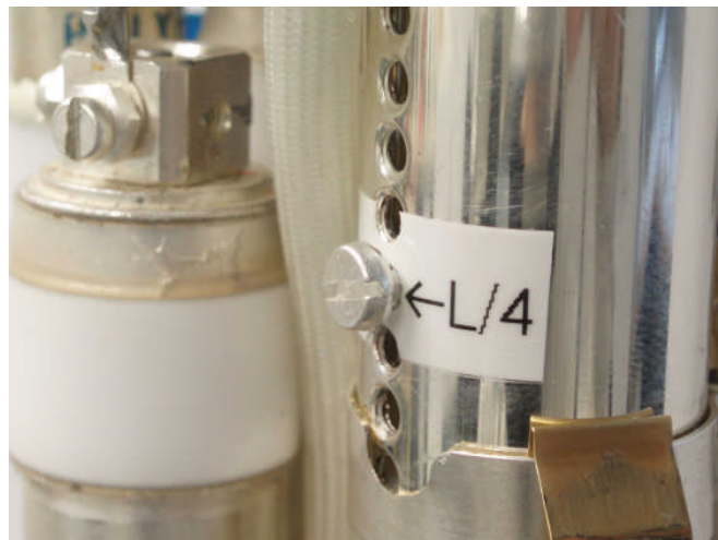
Fig.4 screw in \rightarrow \lambda/4 -mode
