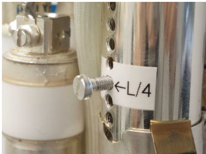
Fig.3 screw out \rightarrow \lambda/2 -mode
