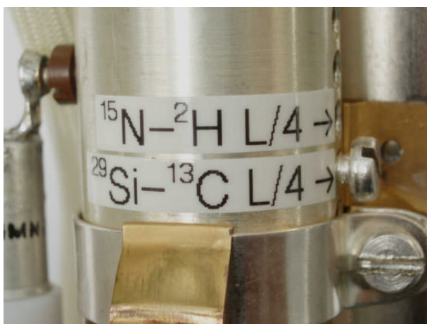
Figure 3: short circuit screw in ^{29}\text{Si}-^{13}\text{C} position
