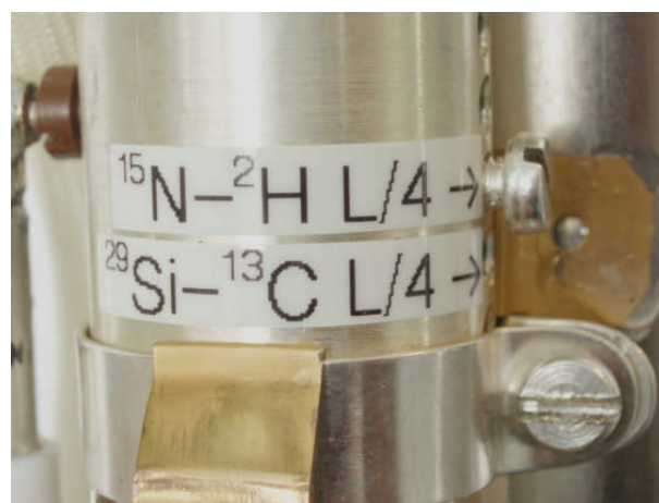
Figure 2: short circuit screw in ^{15}\text{N}-^2\text{H} position
