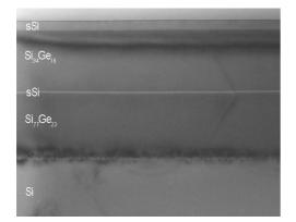
Figure 1 - XTEM image of a strain relaxed Si.77Ge.23 layer overgrown with a strain compensated 200 nm SiGe layer of 16at% Ge. The strained Si cap layer has a thickness of 40 nm.
