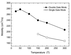
Variation of maximum magnetoresistance mobility with temperature for single gate (squares) and double gate mode (circles)
