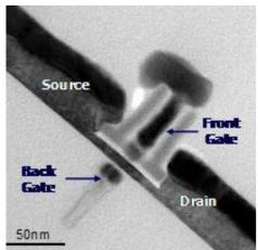
TEM cross-section of the devices tested
