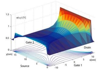
Modeled subthreshold potential distribution for DG MOSFET with applied drain bias
