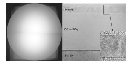
Figure 2 - Left side shows an infrared transmission image of a 200 mm sSi/SiGe wafer bonded to Si using a PE-CVD Oxide as a bonding layer. The right XTEM image of an SSOI wafer shows 18 nm strained Si on 100 nm SiO2 after wafer bonding. The inset shows a magnification of the single crystalline sSi layer.
