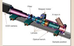
Figure 5: 3D section of the new XEOM, shown with a simple filter carrier The focusing lens can be operated manually or controlled remotely by driving it with a stepper motor. The total length of the system is increased to accommodate the new optics which provide ~12x magnification.
