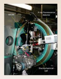
Figure 1 : The XEOM is mounted on the Huber goniometer at beam line BM28 (XMaS) at the ESRF, Grenoble, France.
