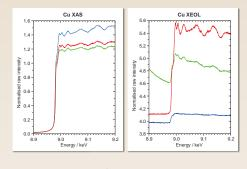
Figure 3: The Ultralene® window appears to increase the background luminescence. This is not seen when the water is introduced; it is possible that the water modifies the modifies the Ultralene®, or even permeates the window.
