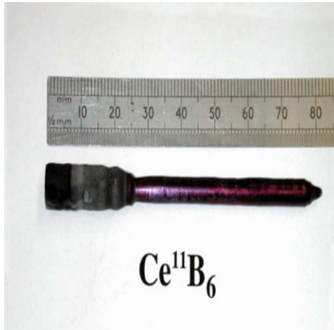
Fig. 1. Photograph of an as-grown boule of \text{CeB}_6 , grown with enriched ^{11}\text{B} isotope for use in neutron scattering studies.
