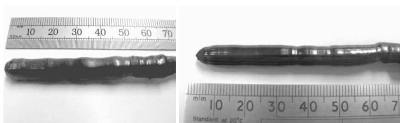
Figure 1. Photograph of the as-grown boules of \text{Ni}_3\text{V}_2\text{O}_8 (left) and \text{Co}_3\text{V}_2\text{O}_8 (right) grown by the floating zone technique.
