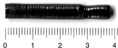
Figure 3. FeTa 2 O 6 crystalline boule grown by the floating-zone method at 1.5 mm h -1 in 1 atm of Ar + 3% H. The crystal is approximately 4 cm in length.
