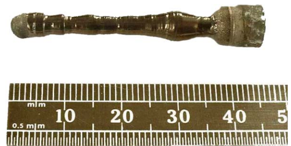
Fig. 1. Photograph of an as grown boule of \text{CrB}_2 obtained by the floating zone technique.
