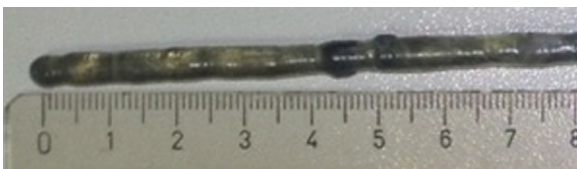
Fig. 4. Photograph of a \text{Ba}_2\text{CuGe}_2\text{O}_7 single crystal grown in this work (batch No. 10).
