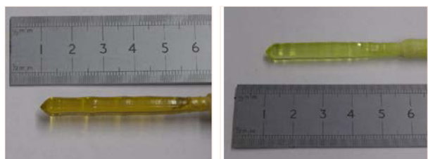
FIG. 2. As grown boules of \text{SrHo}_2\text{O}_4 (left panel) and \text{SrDy}_2\text{O}_4 (right panel) single crystals, using growth speeds of 6 to 8 mm/h. Figure is from Ref. 10.
