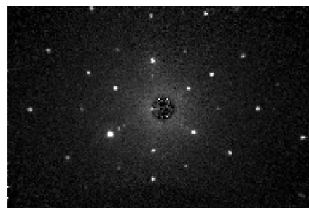
Figure 2. Typical Laue pattern of the as-grown crystal boule. The incident X-ray beam is aligned with the [111] crystallographic direction. The Laue patterns were consistent across the surface of the boule.
