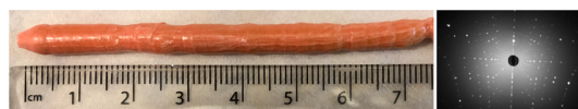
Figure 7. Boule of \text{Ho}_2\text{Si}_2\text{O}_7 prepared by the floating zone method in an air atmosphere, at pressures in the range 1–2 bar, in a flow of air of 0.1–0.2 L/min, using a growth speed of 8 mm/h. Also shown is the X-ray Laue pattern of one of the sides of the \text{Ho}_2\text{Si}_2\text{O}_7 crystal boule.
