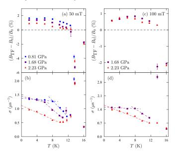
FIG. 6. Measured field shift [(a), (c)] and associated relaxation rate [(b), (d)] extracted from fitting of TF  $\mu^+$ SR measurements of GaV<sub>4</sub>S<sub>8</sub> at different applied pressures and magnetic fields  $B_0$ . Dashed lines in (b) and (d) are guides to the eye.
