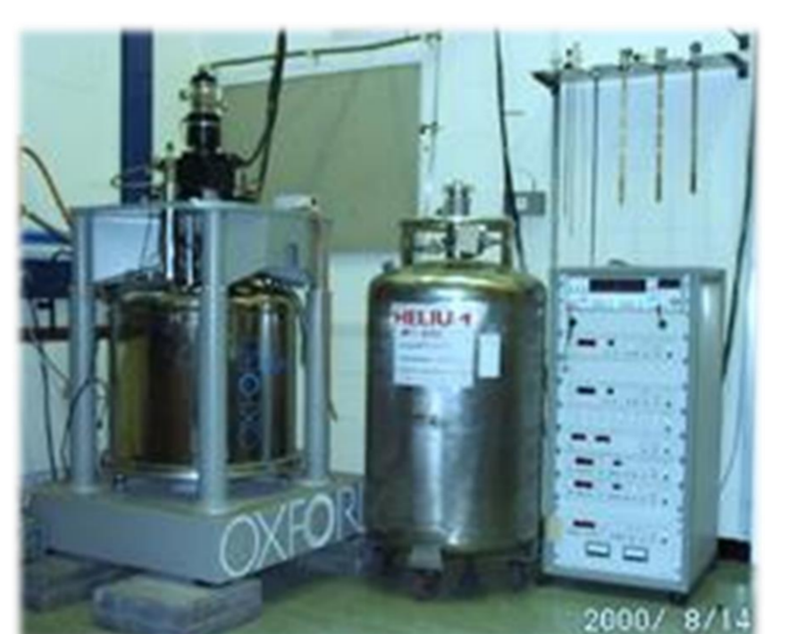
Our 12 tesla Oxford Instruments Vibrating Sample Magnetometer.
