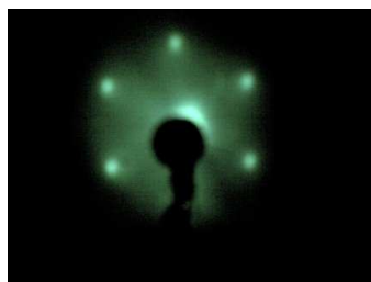
Figure 2.6: Example LEED pattern showing a (1 × 1) reconstruction of a clean InN(000 \bar{1} ) surface.
