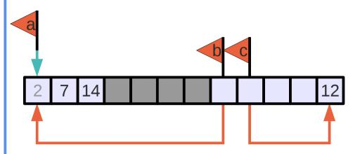
As with pointers, if we increment the variable, we are incrementing the pointer, not the value pointed to
