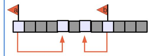
Next, the memory for two integers are allocated and the addresses of these allocations are assigned to the pointers
