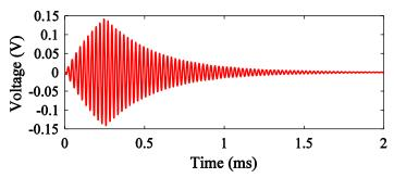
Figure 3: FUT Amplitude-time spectrum from LDV, with a 10 cycle burst at a drive frequency of 40 kHz.
