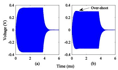
Figure 4: FUT amplitude-time spectra from LDV for drive frequencies of (a) 39.9 kHz, and (b) 40.5 kHz.
