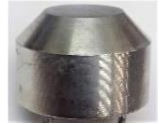
Aluminium FUT, Nominal 40 kHz Resonance in the (0,0) Mode
