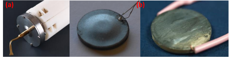
Cymbal-type transducers and devices, for (a) surgery, and (b) tuneable-frequency applications, utilising shape memory alloys
