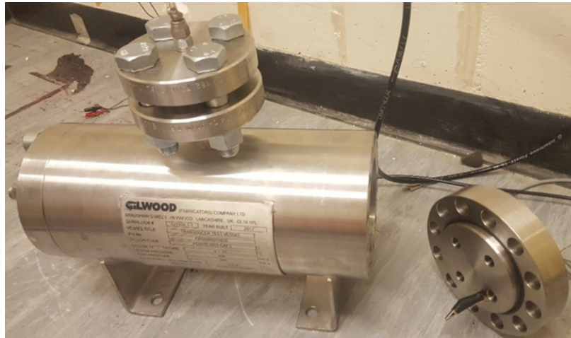
Figure 2.1: The pressurisation system, comprising the pressure vessel manufactured by Gilwood (Fabricators) Company Ltd. connected to the Hill Air Pump.
