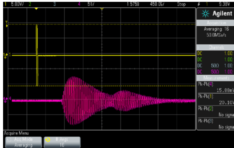
Figure 3.2: Pitch-catch results for two 40 kHz commercial FUTs in the (0,0) mode.
