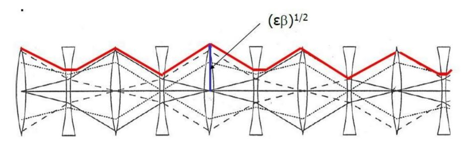
The envelope around all the trajectories of the particles circulatin in the machine is called  $\beta$ -function:
