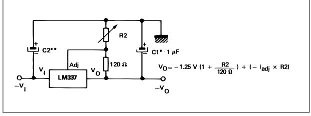
\* C1 = 1  $\mu$ F solid tantalum or 10 $\mu$ F aluminium electrolytic required for stability. \*\* C2 = 1  $\mu$ F solid tantalum is required only if regulator is more than 10 cm from power supply filter capacitors
