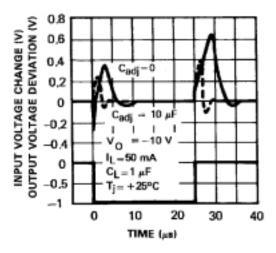
Figure 14: Load Transient Response
