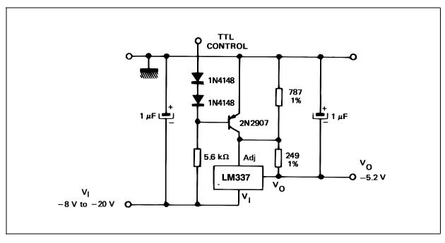
\* Minimum output = - 1.3V when control input is low.
