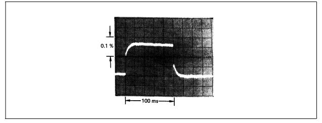
LM337, VO = -10V, V<sub>I</sub> - V<sub>O</sub> = - 40V, I<sub>L</sub> = 0A  $\rightarrow$  0.25A  $\rightarrow$  0A. Horizontal sensitivity 5msN/div.
