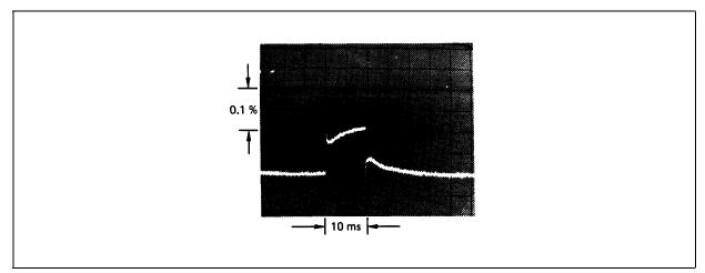
LM337, VO = -10V, V<sub>I</sub> - V<sub>O</sub> = - 40V, I<sub>L</sub> = 0A  $\rightarrow$  0.25A  $\rightarrow$  0A. Vertical sensitivity 5mV/div.
