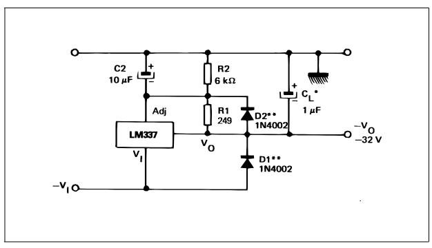
$^*$  When CL is larger than 20  $\mu F,$  D1 protects the LM137 in case the input supply is shorted.  $^{**}$  When C2 is larger than 10  $\mu F$  and VO is larger than -25V, D2 protects the LM137 in case the output is shorted.
