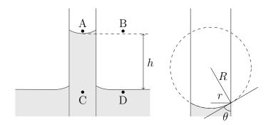
(a) By considering the pressures at points A, B, C, and D in the diagram, construct a pressure balance to derive the following equation for the capillary rise h:
