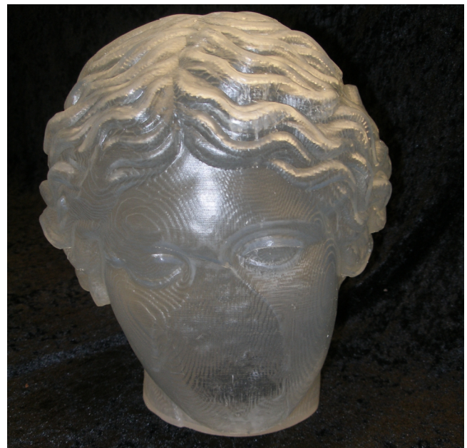
Figure 14: Photograph of the Rapid Prototyping Realisation of the Head.
