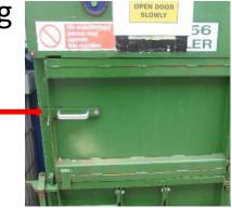
4. Open bale chamber door by pulling lever towards yourself and releasing lower pedal with foot.
