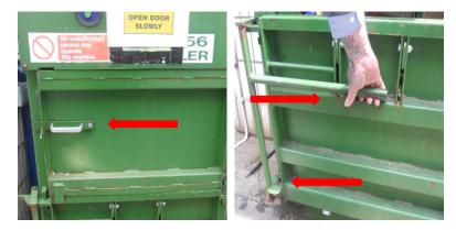
10. Compression head should be in 'down' position. Insert 'strap-hook' through slots located on top of compression head and pull baling tape from rear of baler.
