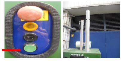
8. Repeat loading and crush-cycle processes until baler is full. **NB:** amber light on control panel will illuminate once baler is full.
