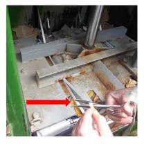
14. Stand clear of baler and press both 'manual' buttons on control panel/lefthand side of baler. This will reset compression head to 'upper' position. **NB:** keep clear of rising compression head.
