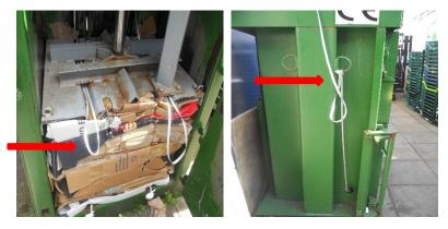
12. Untie baling tape secured to front toggle hooks at front of base. Feed baling tape through loops as shown in Step 11 and tie-off securely.
