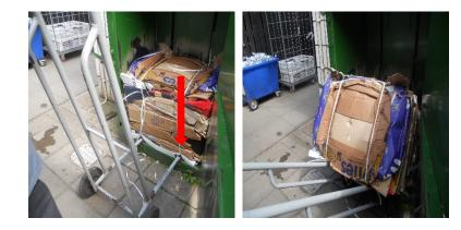
16. Baling tape should be fed along 'feed-channels' to base of baler and ends tied to 'toggle' hooks at front of base. Place flat piece of cardboard on base as this will keep the baling tape in place.
